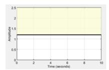
• To specify a single bound with multiple edges, use a two-column matrix. The matrix must be of the form  $[A_1 \ B_1 \ ;...; A_n \ B_n]$ , where n is the number of edges in the bound. For a constant amplitude throughout a time interval, use  $A_k = B_k$ , where k = 1,...,n
