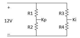
Resistors are commonly manufactured in standard values. Therefore, when using response optimization to identify suitable values for the resistors R1, R2, R3, and R4, it is useful to confine these parameters to a discrete set of readily available resistor values. To do so, use sdo.getParameterFromModel to create param.Discrete parameter objects for each of the resistors. In this case, because all model parameters you plan to optimize are discrete, use [] for the continuous parameters.
